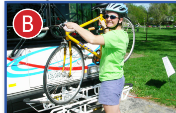
Getting On: Swing support arm up and over
