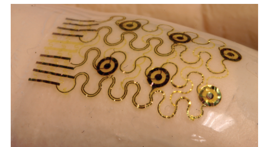
Close-up view of a stretchable circuit applied to the skin
